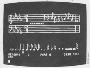
ALF's streamlined menu provides all the necessary notational choices as well as information about current measure and the number of notes that can still be put into memory. The cursor under the menu and the cursor on the staff show that the next note will be a quarternote on F. Placing the cursor over the row of X's at left allows the user to make envelope modifications.
