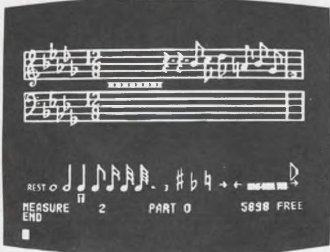
ALF's streamlined menu provides all the necessary notational choices as well as information about current measure and the number of notes that can still be put into memory. The cursor under the menu and the cursor on the staff show that the next note will be a quarter note on F. Placing the cursor over the row of X's at left allows the user to make envelope modifications.
